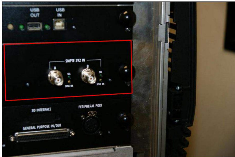
Figure 3: Remove interface board from Barco Projector
