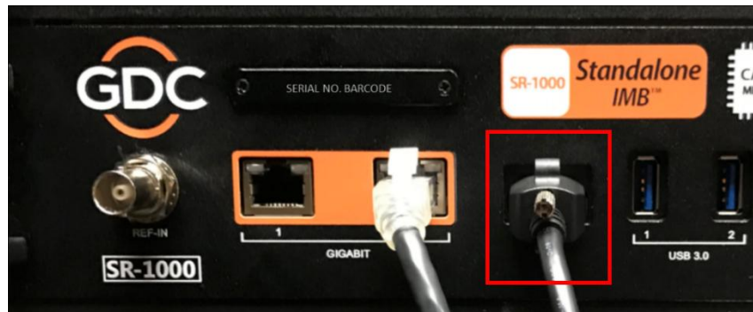
Figure 11: Insert eSATA cable into SR-1000 eSATA port
