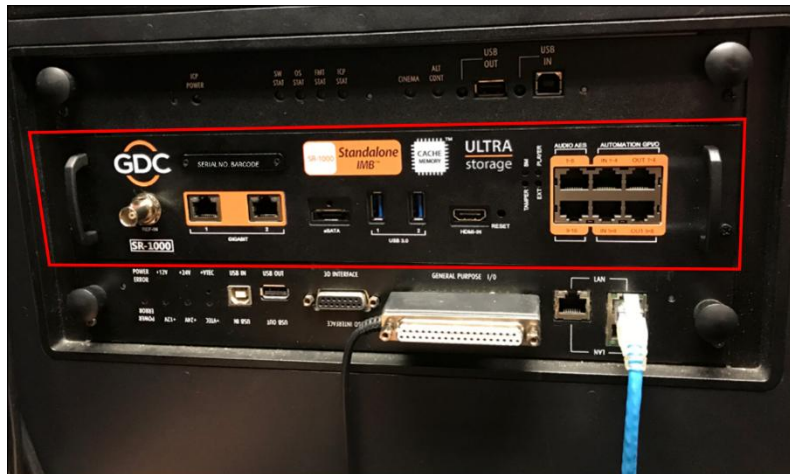
Figure 7: Installing the SR-1000 into the Projector
