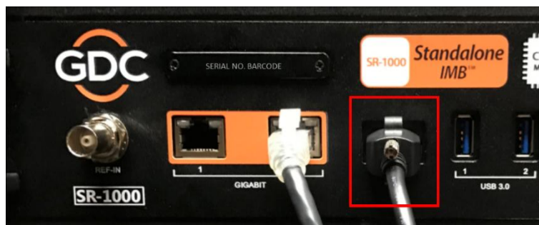
Figure 9: Insert eSATA cable into SR-1000 eSATA port
