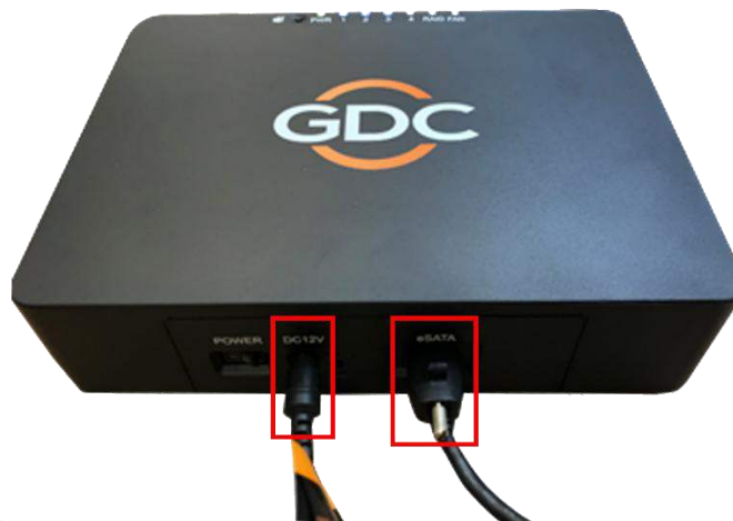
Figure 8: Connect eSATA cable to the Portable Storage
