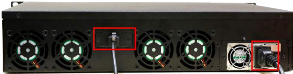
Figure 10: Connect eSATA cable to the Enterprise Storage
