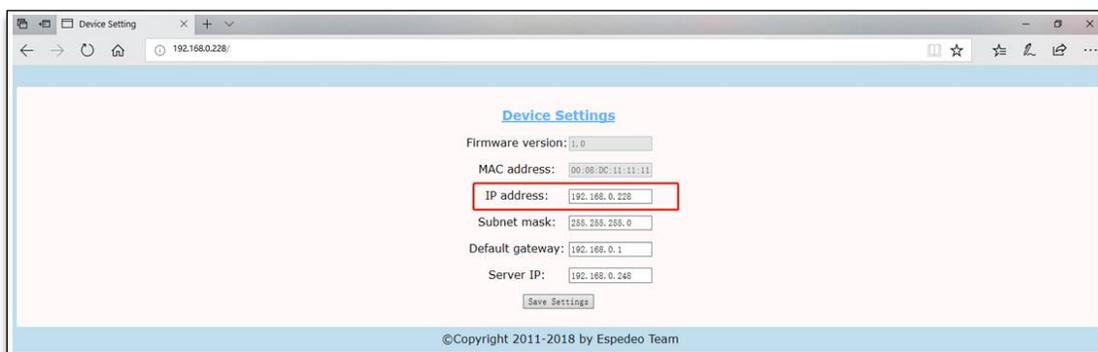
**Figure 18: Verify whether IP Address has changed successfully**
