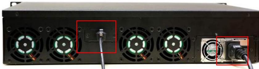
Figure 14: Connect eSATA cable to the Enterprise Storage
