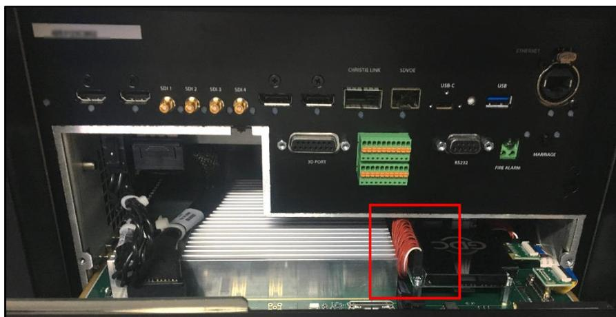
Figure 12: Height of Red Cable on IMB
