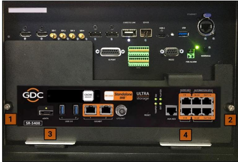
Figure 13: IMB installed in Projector
