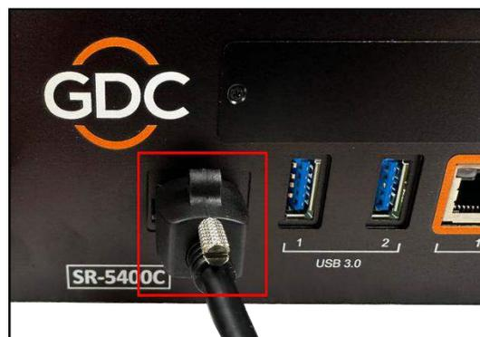
Figure 15: Insert eSATA cable into SR-5400C eSATA port
