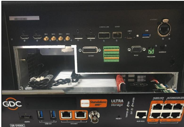
Figure 10: Slide IMB into Projector
