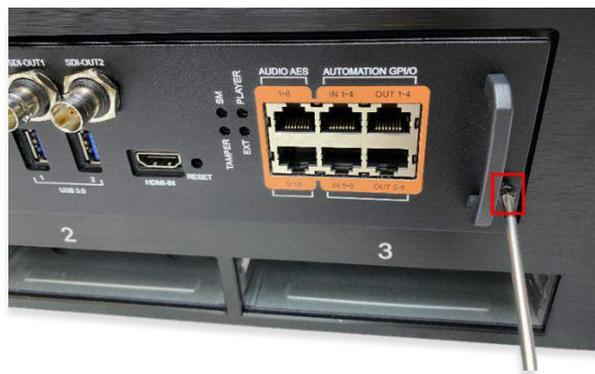
Figure 12: Tighten screws on IMB faceplate
