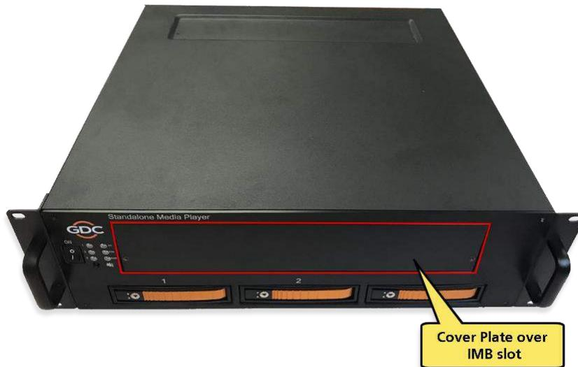
Figure 7: Cover Plate over IMB slot
