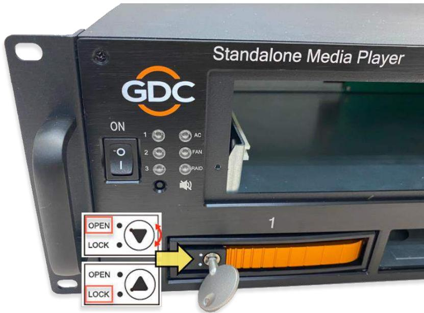
**Figure 6: Lock HDD using Tray Key**
