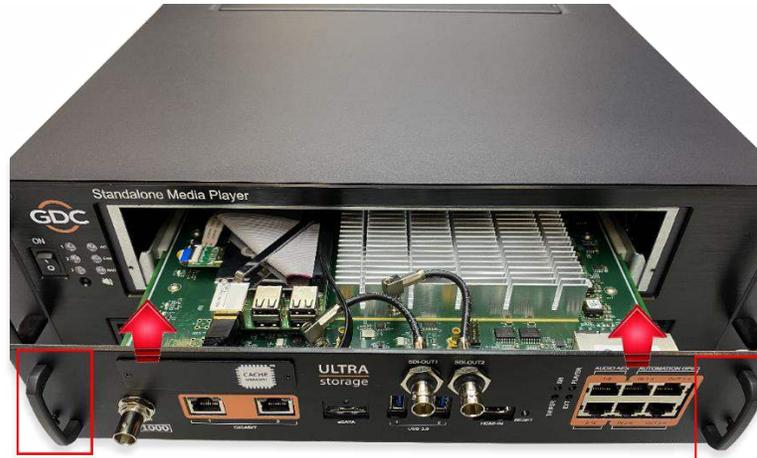
Figure 11: Insert IMB into chassis
