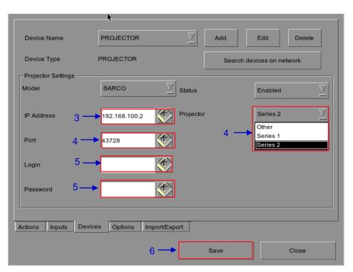
Figure 41 Automation settings for projector device.
