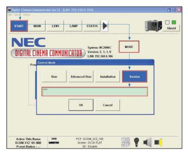
Figure 23 Service Mode on NEC Digital Cinema Communicator.
