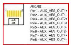
Figure 58 AUX AES Pinout
