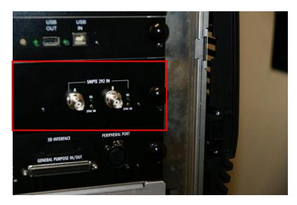
Figure 3 Remove interface board from Barco projector.
