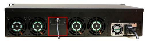
Figure 11 Connect the eSATA cable to the Enterprise Storage
