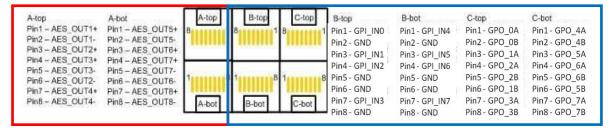
Figure 58 AES audio and GPIO Pinout
