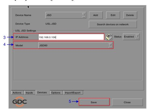
Figure 56 Automation settings for USL JSD device.
