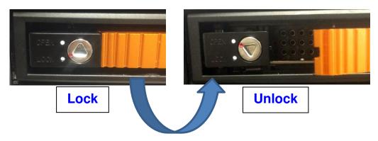
2. Push the 'OPEN/LOCK" icon to release the handle and pull out the HDD tray.
