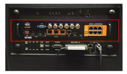
Figure 7 Inserting SX-4000 into the projector.
