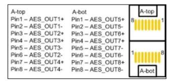
Figure 38 AES Audio RJ45 pinout.
