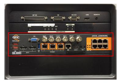
Figure 6 SX-4000 Placement on NEC projector.
