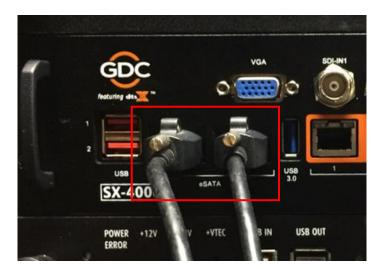
Figure 14 Insert the eSATA cable into SX-4000 eSATA port 2.
