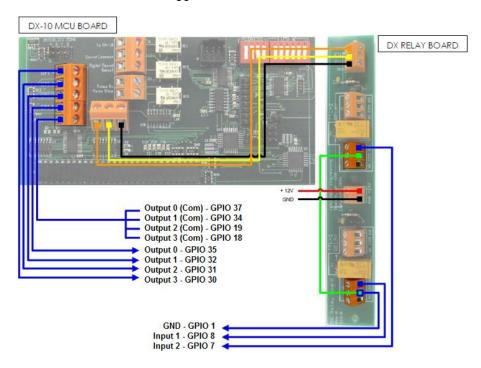
Figure 57 Component Engineering TA-10 wiring diagram.
