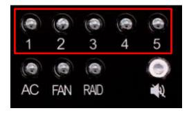
The lights have two colors; Blue and Red. The LED lights can change from steady to flashing depending on the status of the hard drive.
