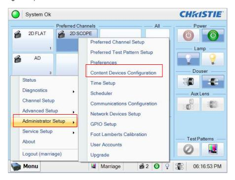
**Figure 27 Content Devices Configuration**
