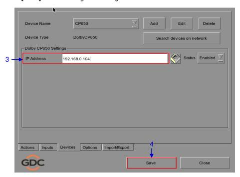
Figure 52 Automation settings for Dolby CP650 device.
