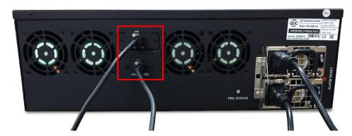
Figure 12 Connect the eSATA cables to the Enterprise Storage Plus
