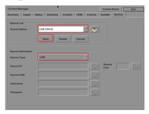
Figure 32 USB ingest source setup.
