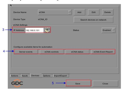
Figure 44 Automation settings for eCNA device.
