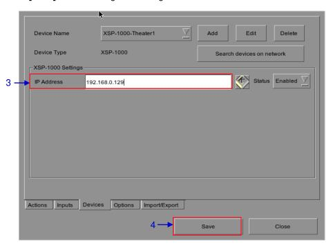
Figure 50 Automation settings for GDC XSP-1000 cinema processor
