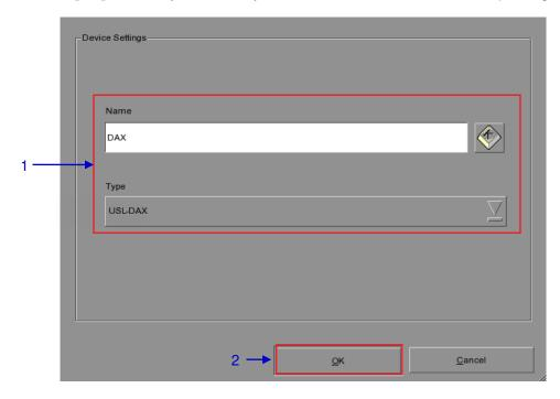
Figure 53 USL DAX automation device setup.
