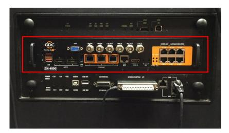
Figure 4 SX-4000 Placement on Barco projector.
