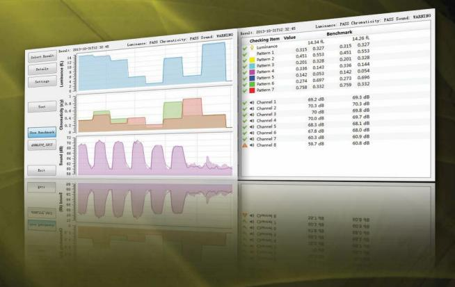
**G** QMS-1000 Quality Management System is designed for cinema screening quality monitoring and control. It manages the quality of projection and audio by measuring and analyzing the luminance, chromaticity and sound pressure level.
