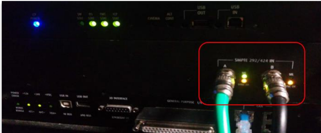
Figure 11: HD-SDI Cables connected to link decryptor board of Series 1 Projector
