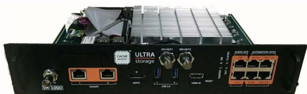
Figure 2: SR-1000 Media Block with HD-SDI Connectors
