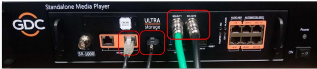
Figure 10: Cable connections on the SR-1000 Standalone Media Player
